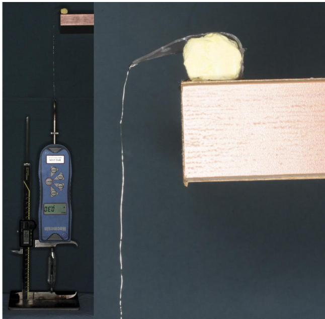
FIGURE 6. Design for a measuring tool for a force gauge fixed with a micrometer. A screw was welded between the arms of the micrometer. The micrometer and posterior side of the force gauge were welded. The force gauge was moved up and down along the screw. The force applied to the PLLA sheet or Medpor (porous polyethylene) was measured with the force gauge, and the degree of sagging was also measured with the micrometer. Left, Force and degree-of-sagging experiment. Right, Magnification of the model of the orbital floor reconstruction.
